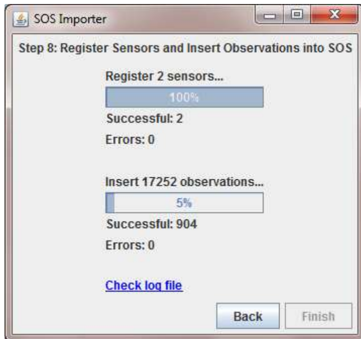
Step 8: Registering sensors and inserting observations at the specified Sensor Observation Service
